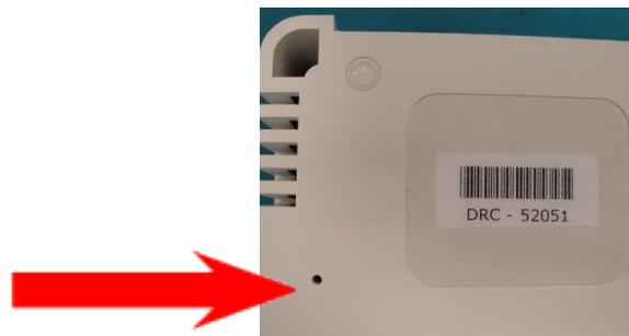
2. Once the DRC-300 has been reset, go to Step 9 of this section.
