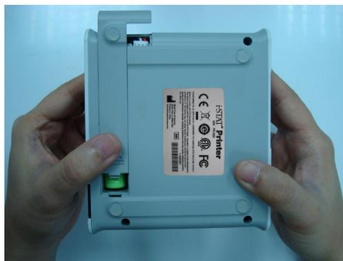
3. If replacing an existing rechargeable battery in the printer, disconnect the existing battery by gently pulling up on the red/white/black wires until the connector releases from the three metal pins. Once the battery is disconnected, remove it completely from the battery compartment.
