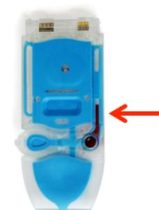
These images display under-filled cartridges. In the images on the left, the sample well is insufficiently filled, and the sample does not reach the fill mark indicator.
