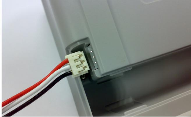
6. Slide the connector onto the three metal connector pins.
