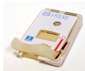
These images display improperly closed cartridges. Although they were properly filled, they must be closed sufficiently before they may be inserted into the device.
