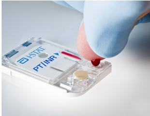
**Note:** To further simplify the sample application into the test cartridge, it is possible to bring the cartridges to the finger for easier application. Do ensure that the instrument remains on a flat, vibration-free surface for testing
