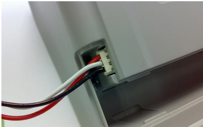
7. Once the wires are connected, place the battery portion of the pack into the rectangular compartment. Make sure the wires are not under the battery or projecting out of the opening. The correct positioning is shown below.
