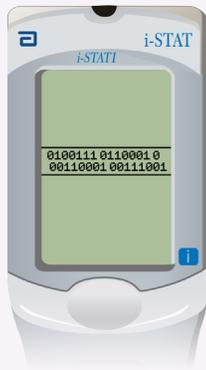
Do not move the analyzers until the Sending Analyzer goes back to the Utility menu, and displays **Last Send Successful**. The update is now complete.
