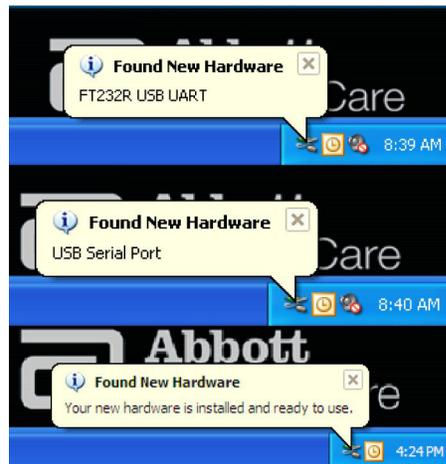
6. Select **Start → Settings → Control Panel → Performance and Maintenance (if listed) → System** to launch the “System Properties” dialog box. Select the **Hardware** tab and click **“Device Manager”** to show a list of devices.
