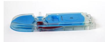
These images display a properly filled cartridge. In the images at the top, the sample fills the sample chamber to the fill mark indicator.
