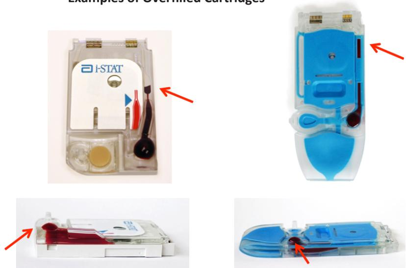
These images display overfilled cartridges. In the images at the top, the sample exceeds the fill mark indicator. In the images at the bottom, you will notice a bubble in the sample well.
