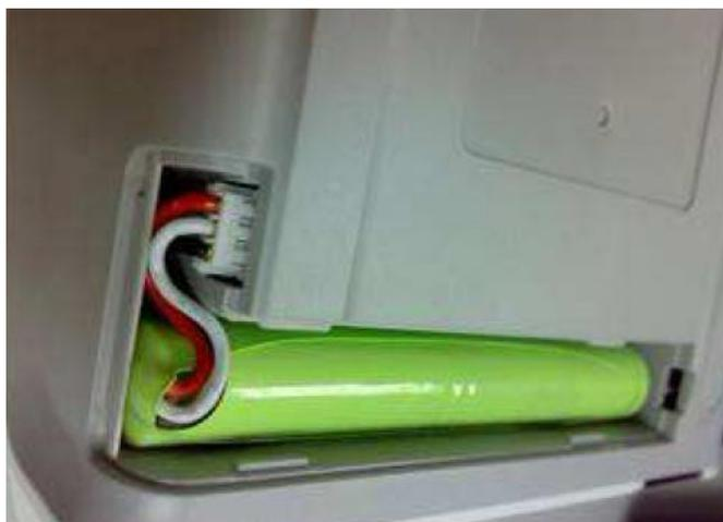
8. Slide the battery door back onto the compartment until it closes and locks into place.
